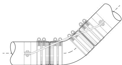
**2. STEPPED JOINTS:** When two pieces of pipe come together, they are never the exact same outer diameter due to +/- tolerances. A thinner shield is more forgiving, flexible and malleable. It bends with the joint allowing the seal to remain strong. A thick shield is rigid and does not form itself over the joint.
