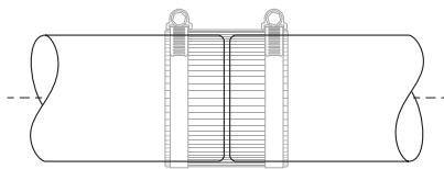
**1. TRANSFERENCE OF TORQUE:** Thicker gauge shield material "blocks" the torque from getting to the gasket. A thinner shield protects the gasket while allowing a more efficient transfer of torque therefore providing a better seal.
